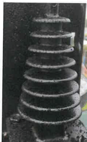
Insulator on coal-wood fire, second monitoring round, 27 June
